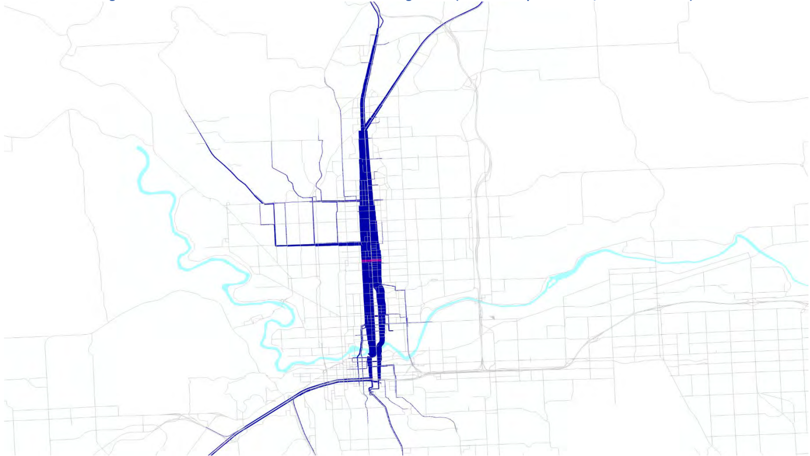
Figure B6: No Build AM Peak Period Flow Bundle for Segment 3 (North of Empire Avenue/Garland Avenue)
