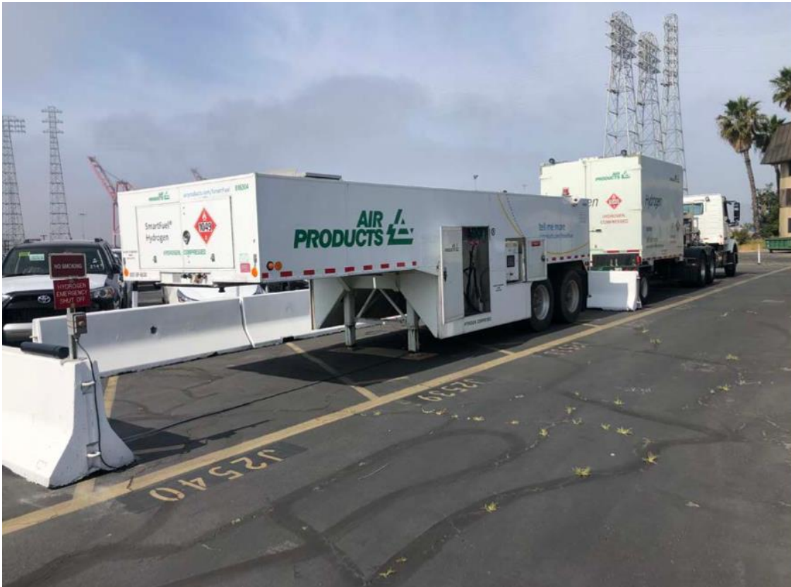
Figure 33: Mobile Hydrogen Fueling Trailer
