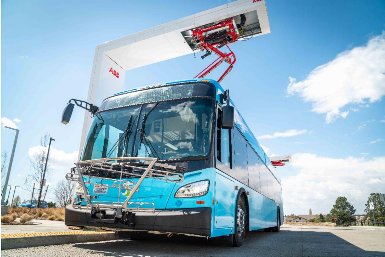
Above: An STA battery-electric bus being charged at an overhead pantograph charger at Moran Station Park & Ride
